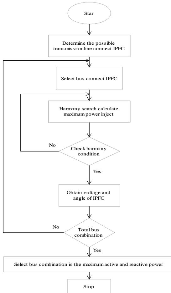
Figure5 flowchart of optimal location IPFC using HS
