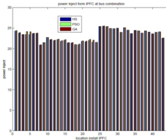
**Figure8** Power inject of IPFC at various position in the system
