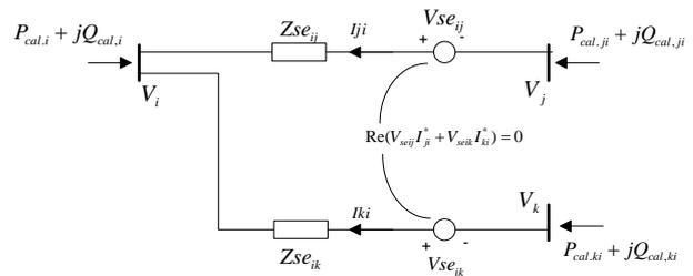
**Figure 3** Equivalent circuit of IPFC
