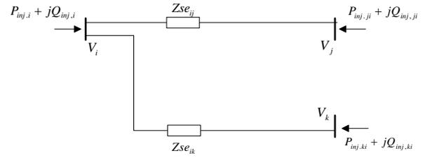
Figure4 Injection model of IPFC
