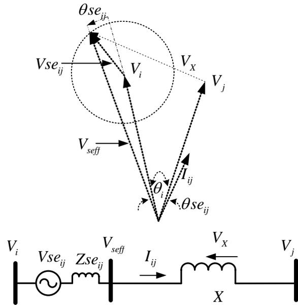
**Figure 2** Phasor diagram of voltage control
