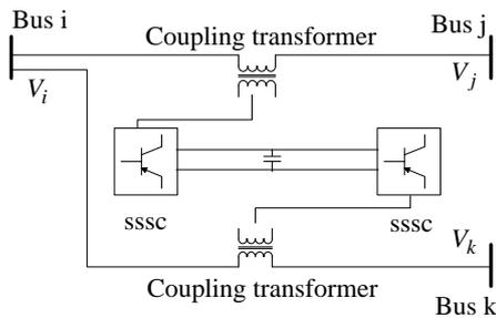
**Figure 1** Schematic representation of a two converter IPFC
