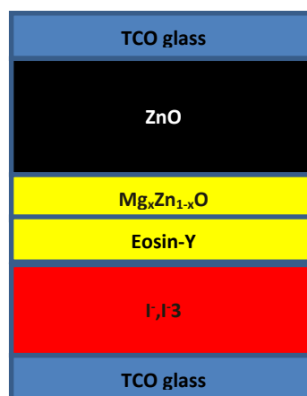
Figure 1 Schematic diagram of DSSC structures used in this experiment.
