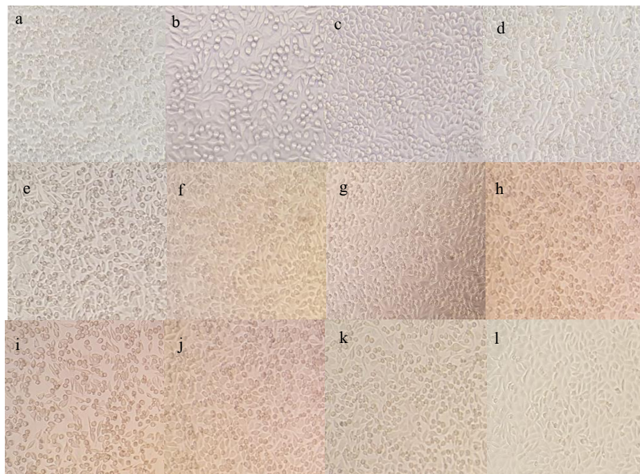
Fig.4. Cell morphology in MEM elution assay of 0.2 g/ml extract from blood bags of manufacturer A (a-AS-5, b-CPD bag, c-platelet bag, d-satellite bag), from blood bag of manufacturer B (e-RBC Bag, f-CPD Bag, g-Platelet I bag, h-Platelet II bag), and from blood bag of manufacturer C (i-AS-5 bag, j-CPD bag, k-Platelet I bag, l-Platelet II bag)
