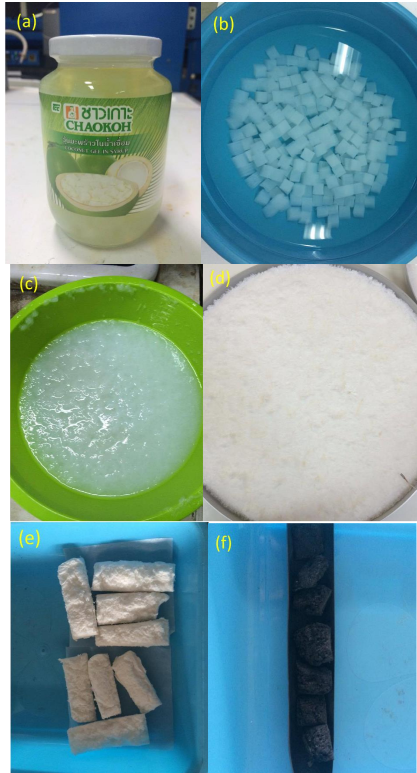
Figure 1 Processing of BC: (a) as-purchased BC in the form of Nata de coco (Coconut gel in syrup, Chao Koh), (b) BC soaked in water to remove syrup, (c) BC after blending, (d) BC after freeze-dried, (e) FD-BC cut into pieces, (f) carbon nanofiber obtained from the pyrolysis of FD-BC.
