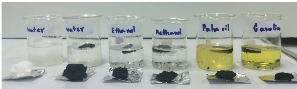
Figure 6 Liquid absorption experiment. From left, FD-BC soaked in water, carbon nanofibers from pyrolysis of FD-BC soaked in water, ethanol, methanol, palm oil and benzene (gasoline).
